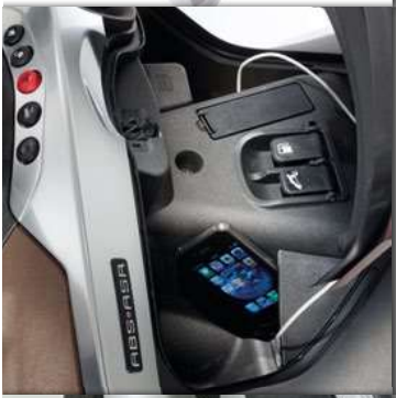
The large leg shield back plate features two lateral compartments and a central compartment with a 12V power outlet.
