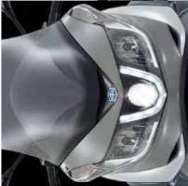
Poly-elliptical full beam headlamp with LED strip daytime running light
